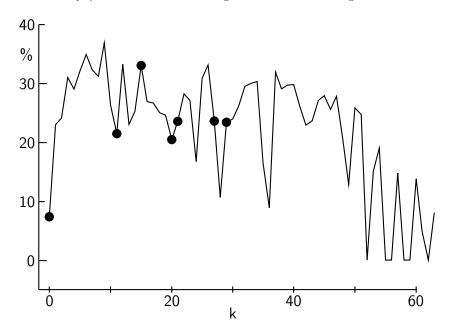
Figure 4. The percent reduction of perceptual error achieved by the artifact reduction system. Zero percent corresponds to  $Q_s$  error values, one hundred percent corresponds to  $Q_e$  error values. The dots indicate networks trained with the constant divisor training method; for all other coefficients, the cross-validation performance of a network trained with the constant error method was superior.
