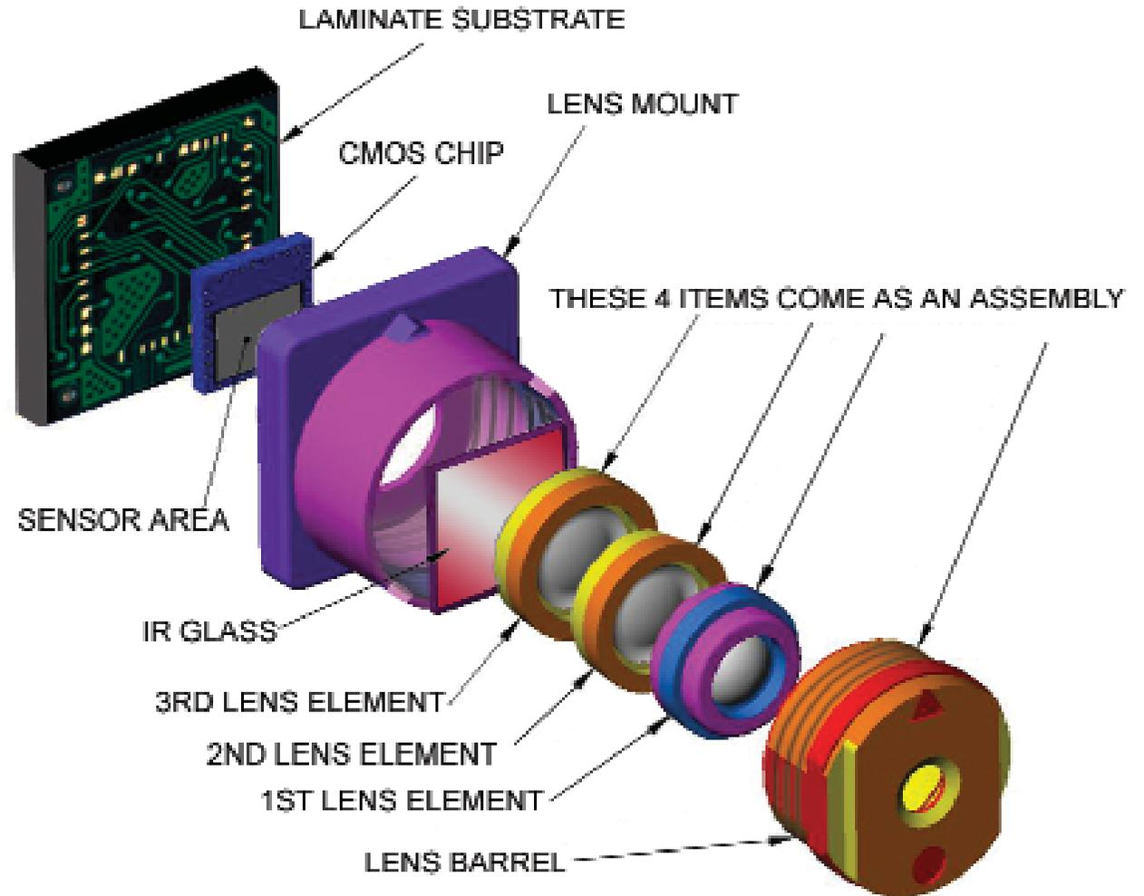
**Camera Module Exploded View**
