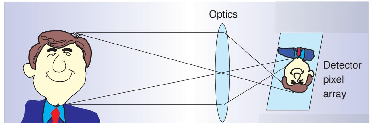
$5\mu\text{m}$  pixels match the optical resolving power of practical camera optical systems (1997, Fossum).
