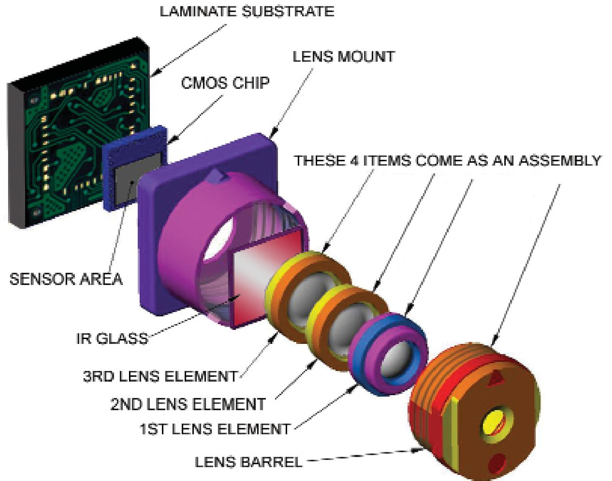
**Camera Module Exploded View**
