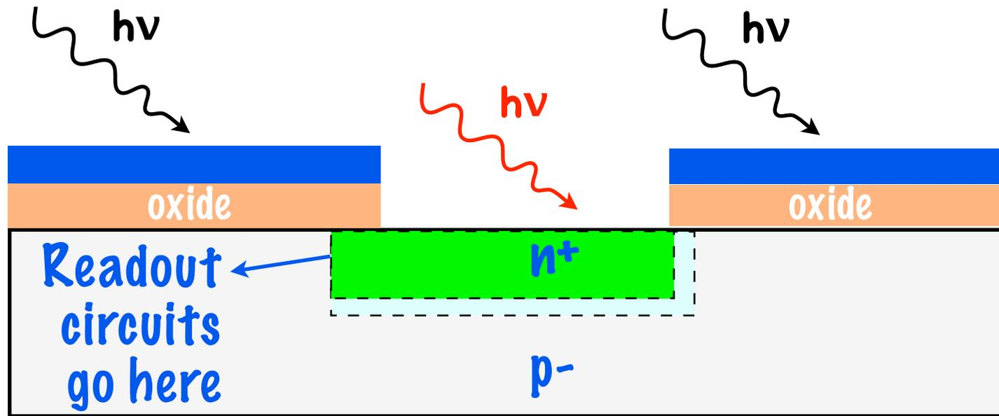
$$\text{Fill factor} = \frac{\text{Photodiode area}}{\text{Pixel area}}$$
