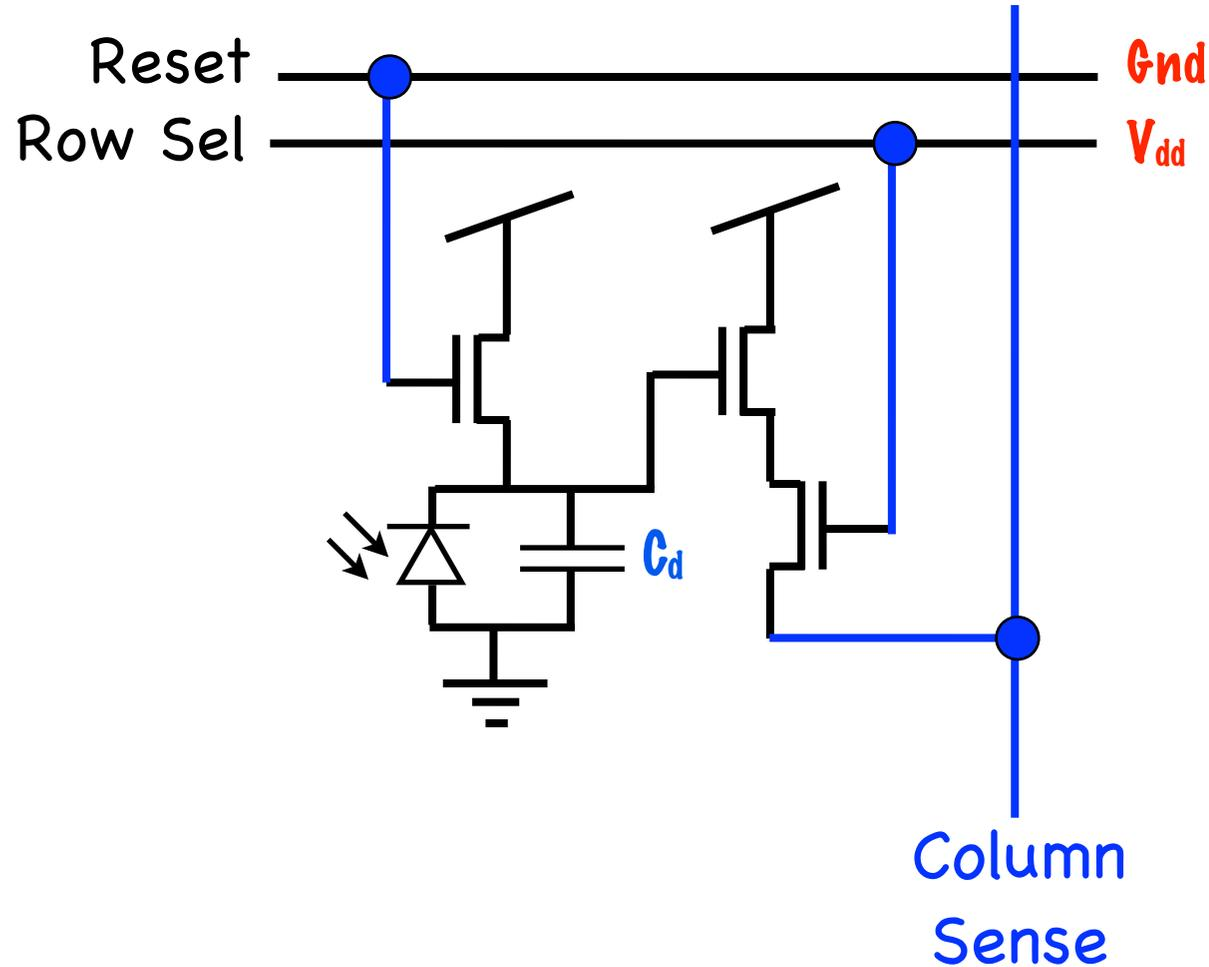
Use  $I(Q_f)$  from start of the cycle to reduce  $kTC$  (reset) noise.
