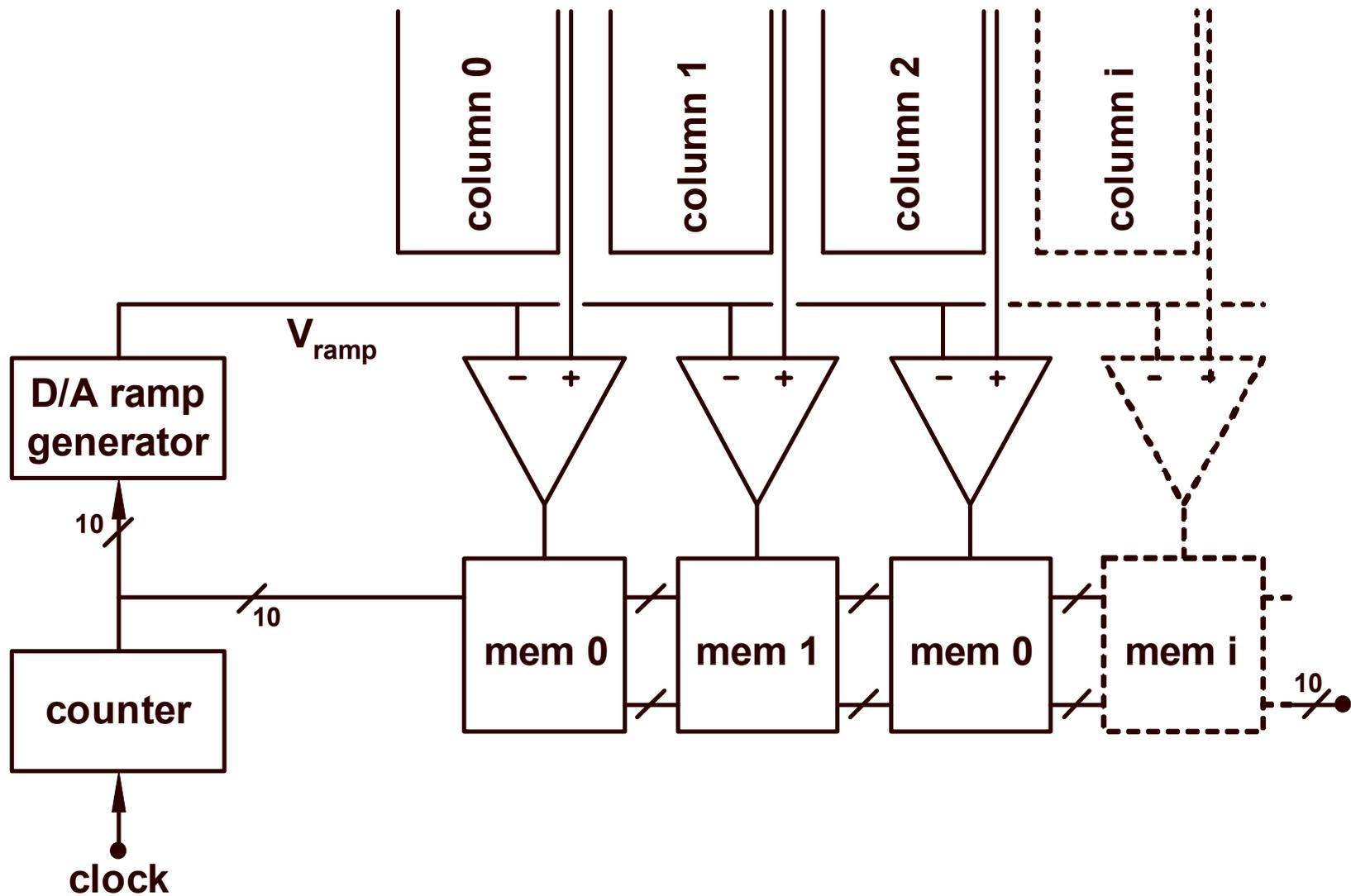
Figure 7. Basic architecture of a column-parallel, single-slope analog-to-digital converter.
